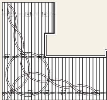
I start by overlaying my design on a deck plan with standard 12-in.-on-center joist framing.
